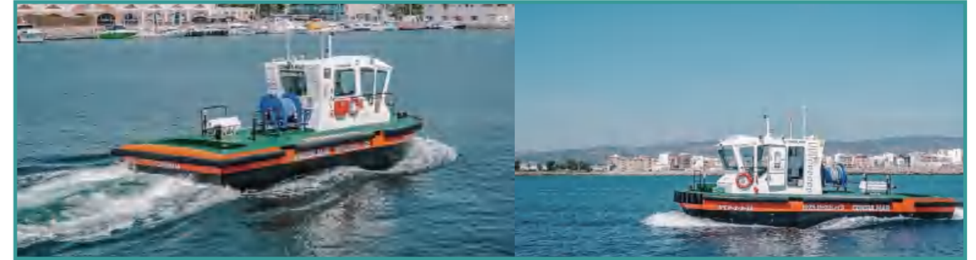
Powered Spain's first electric boat (13M, 60T) with our propulsion system and EVE battery.
