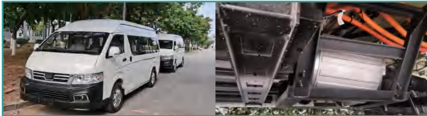
Implemented a direct-drive powertrain system in vans.
