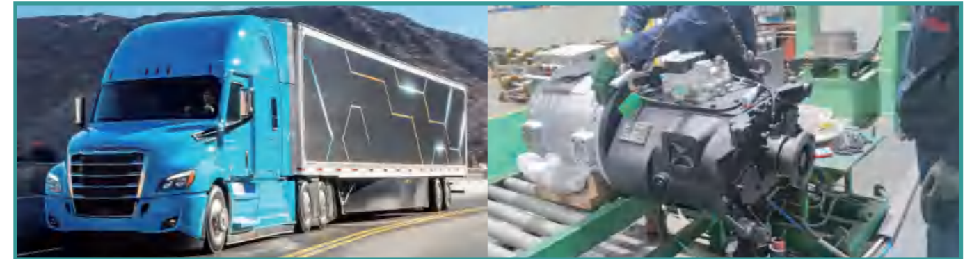
Developed a 40-ton semi-truck prototype in India, integrating a 350KW motor with a fast 6-speed gearbox.
